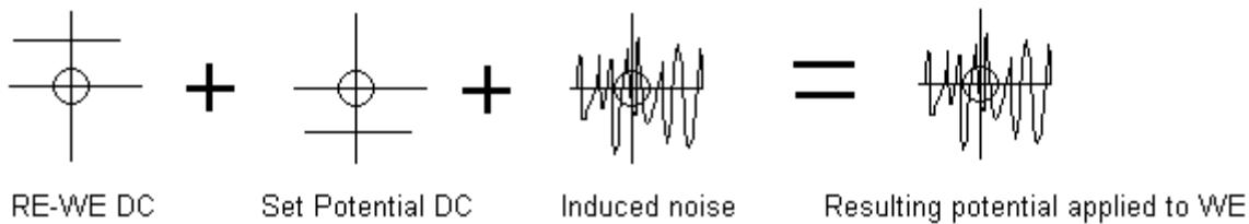
At ACM we have discovered that the way to solve the problem of induced pickup is to provide an AC coupled low impedance path between the input of the reference electrode buffer and the bulk electrolyte. This path is easily achieved using an ACM Noise Reducing Electrode as a fourth electrode in the cell. Because this electrode is AC coupled the DC component of the reference is not effected.
