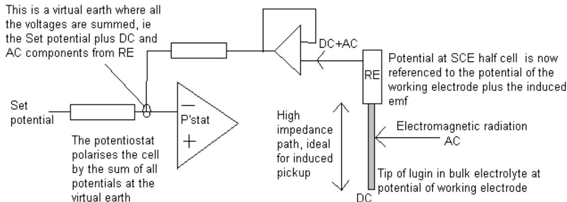
The electromagnetic radiation has two components the easily screened out electrical component and the much more difficult magnetic component. It is the magnetic component that penetrates Faraday cages and causes problems even in well screened systems.
