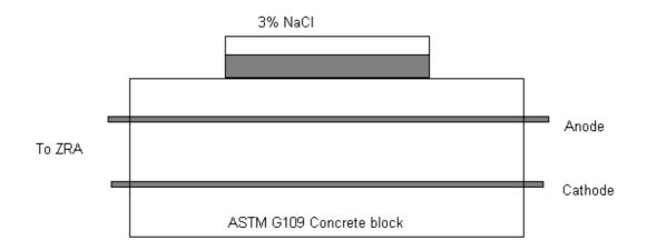
This test block can also be used to measure IR compensated LPR and AC Impedance by applying a test frequency from 10000 Hz to 1 mHz mechanistic information of the corrosion processes can be obtained by studying the time constants revealed. Some workers have used a galvanostat (e.g. Gill AC in galvanostat mode) and pulsed the concrete with known amounts of charge the potential change is then recorded and the time constants of the cell calculated.
